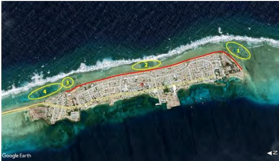
Figure 5-13: Borrow pit groupings (highlighted in yellow) in relation to the seawall alignment (red).
