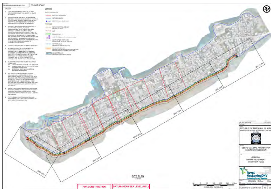
Figure 2-2: Proposed seawall alignment (in orange) 10
