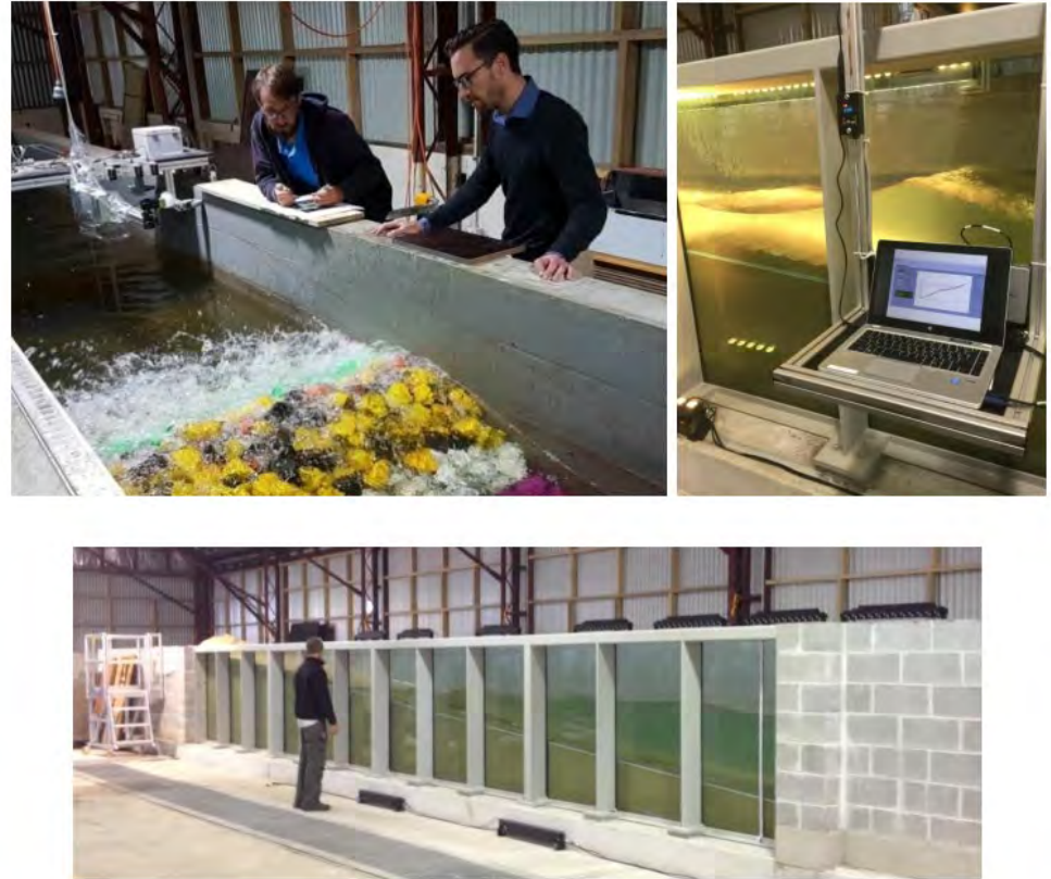
Figure 1: 1.2 m wide wave flume facility
